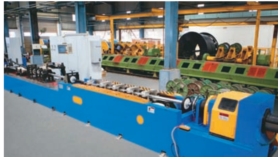
Aluminium Corrugation Sheathing Line
