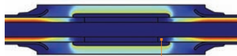
Simulations: Design based on computer FEM-simulations for optimal electrical stress.
