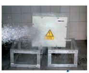
Test object during the water jet test - no water recognized inside cover and housing.
