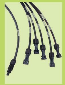
PV String Harness are produced in a dual molding procedure. This guarantees a long product life-time. Through pre-molding maximum impermeability is achieved. Then, final molding guarantees outstanding mechanical properties and high temperature resistance. The cables are pre-assembled according to customer requirements & designs so that it can connect quickly and easily at site. These harness can be manufactured & available in various cable cross-section between 2,5 mm², 4 mm², 6 mm² and 10 mm².
