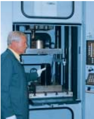
For silicone joints. Extrusion machine for the manufacture of pre-moulded slip-on silicone-insulating bodies and stress cones.
