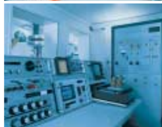
Test room. Routine testing of every length of cable. Test room of alternating voltage and partial discharge test field.
